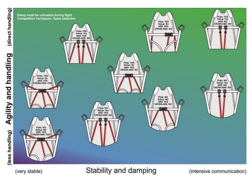
Fig. 11 Overview of different harness geometries and damping
