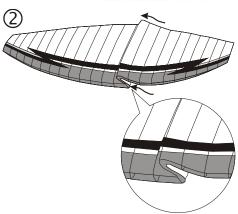
Next, all the ribs on one side are placed one on top of the next, so that the leading edges are not bent.
