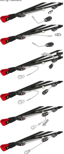
Fig. 9 Installing the speedlimiter
